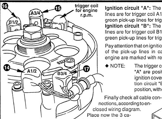
Ignition circuit "A": The yellow-blue pick-up lines are for trigger coil A1/2 @ and the whitegreen pick-up lines for trigger coil A3/4 (5). Ignition circuit "B": The yellow-blue pick-up lines are for trigger coil B1/2 6 and the whitegreen pick-up lines for trigger coil B3/4 7.
